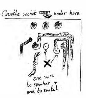
Solder the capacitor and the two resistors to the switch, as shown in the illustration, and run a length of wire from the capacitor to either one of the contacts X on the main board, behind the cassette take-off socket. •ne of the speaker wires is then taken to the other X terminal, and soldered in place.
