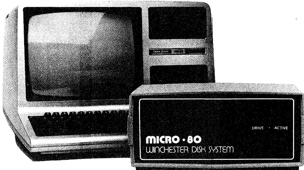
MICRO-80 fits reliable MPI disk drives to the TRS-80 Model 3 to give system capacities and capabilities far in excess of those available elsewhere. All our conversions utilise low dissipation, switching-mode power supplies to avoid screen jitter and overheating. The disk controller boards used incorporate special compensation circuitry for 80 track disk drives and may also be used to run 8 inch disk drives with an appropriate cable and DOS.
