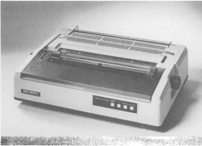
A daisy wheel printer which produces sharp, clean copy suitable for word processing.
