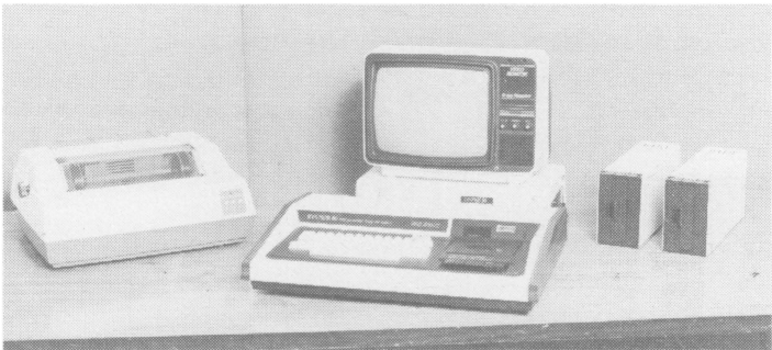
A System 80 set up with quite a few peripherals including an expansion unit, two disk drives and a dot matrix printer ... all discussed and explained in this chapter.
