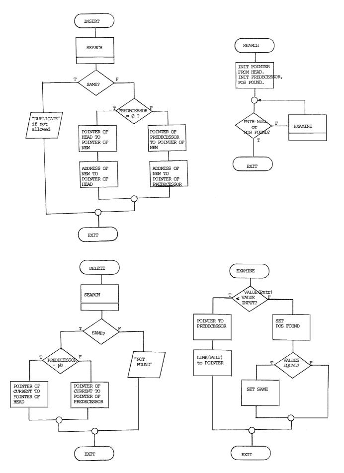
FIGURE 2 - General processing algorithms - singly linked linear lists. Note: Pntr is an abbreviation for POINTER APPLYING THE NEW DATA STRUCTURE.
